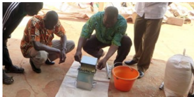
Figure A2 | Example of a “Riffle Divider”
