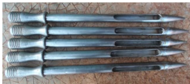
Figure A1 | Example of a “Spear Sampler”
